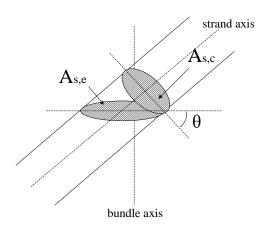
Fig. 3. In the cross section of the bundle the strand cross section becomes elliptical.
