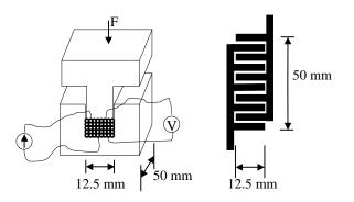
Fig. 5. Experimental apparatus for measuring the interstrand resistivity. Adjustable force can be applied such that the effect of pressure on the interstrand resistivity can be taken into account. The right side shows the interdigitated electrodes. These electrodes were placed on the top and bottom of the rectangular region where wires were packed. With these electrodes, contact resistance between electrodes and strands will not be included in the measurement.
