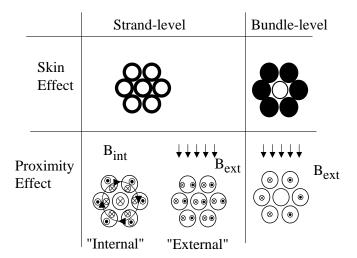
Fig. 1. Types of eddy-current effects in bundled wire.
