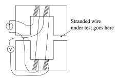
Fig. 7. Experimental apparatus used to measure proximity effect eddycurrent loss in stranded wire. Two windings are used, as in a standard coreloss measurement, such that the measurement (performed with an impedance analyzer) does not include loss in these windings. However, the measurement does include eddy-current loss induced in a wire sample placed in the gap. The windings have a total of ten turns each, five on each core-half (Ferroxcube U93/76/30 size of 3C85 ferrite).
