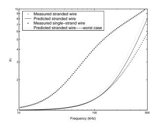
Fig. 6. Experimental ac resistance factor  $F_r = R_{ac}/R_{dc}$  for a transformer wound with stranded wire with 66 uninsulated 40 AWG strands, or with 22 AWG solid wire. Compared with a solid-wire winding, a stranded-wire winding provides a great loss reduction. Our model predicts the loss in stranded wire with high accuracy up to 100 kHz and reduced accuracy up to 500 kHz.
