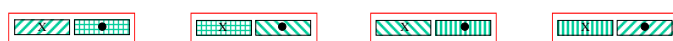
Fig. 6. Schematic of the cross-sectional view of the microfabricated coupled inductors. Eight conductors constitute four single-turn windings, each represented by a similar shade. The four larger rectangles represent the cores. The direction of the conductor dc current into the plane of the page is shown by an X and out of the plane of the paper is shown by a •.
