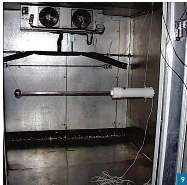
An experimental test of deicing a 1-m line. The suspended bar, 25.4 mm in diameter, was coated with 7 mm of ice for the test. The large-diameter white cylinder on the right contains the resonant inductors submerged in oil.
