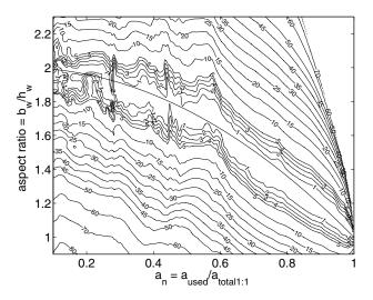
Fig. 3. Optimum winding window aspect ratios based on the simple 2-D analysis, as in Fig. 2, but with contour lines added to show the percentage of winding loss increase from the optimum.
