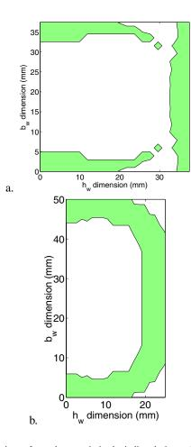
Fig. 1. Comparison of two shape-optimized winding designs with different window aspect ratios. Both are for a 50 kHz 0.5 A rms current in a 100-turn litz-wire winding using 36 AWG (0.127 mmm) strands. a. (top) Winding loss = 133 mW. b. (bottom) Winding loss = 109 mW. Wire is placed in the shaded area. The gap is in the middle of the left side.
