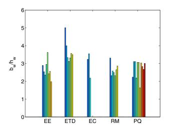
Fig. 6. Typical core aspect ratios  $b_w/h_w$ . Optimal values range from one to two, as shown in Figs. 2 and 3.
