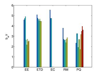
Fig. 7. Typical core aspect ratios  $b_w/r$ . A value of 0.5 is optimal for most designs. As shown in Fig. 4, values around one are almost as good, but losses increase with higher aspect ratios.
