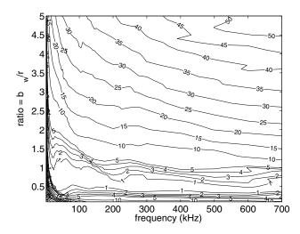
Fig. 4. Optimum ratio of window breadth to centerpost radius, showing percentage winding loss increase from the optimum. The vertical scale is applicable to any design, whereas the frequency scale would shift for other example. The example ploted here used strand diameter d=0.1 mm, packing factor  $\mathrm{F}_p=0.85$ , and radius  $\mathrm{r}=10$  mm.
