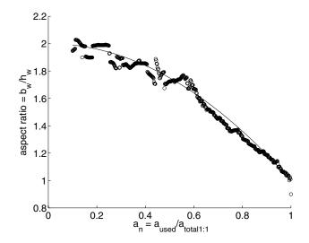
Fig. 2. Optimum winding window aspect ratios based on the simple 2-D analysis. The numercial results (circles) are shown with a curve fit (2) to these results.
