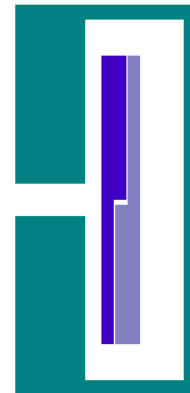
Figure 4: A 2D model modified to have the same reluctance as the 3D model.
